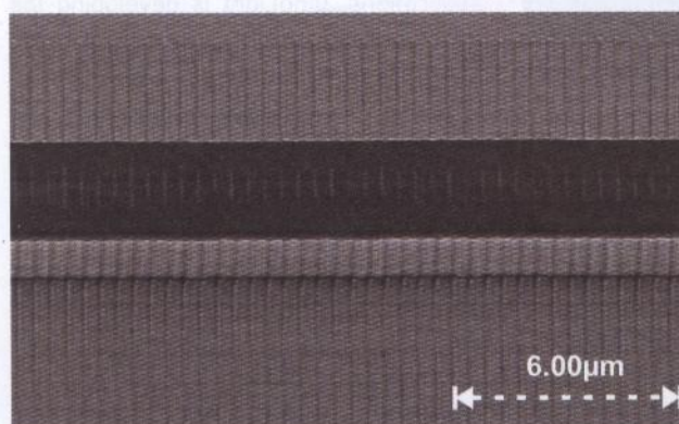
2 DFB laser: ridge waveguide with lateral metal grating (left), and the laser covered with thick gold layer (right)
